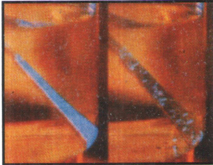
Ultraseal Sealant washes away easily from the surface of an aluminium test piece.
